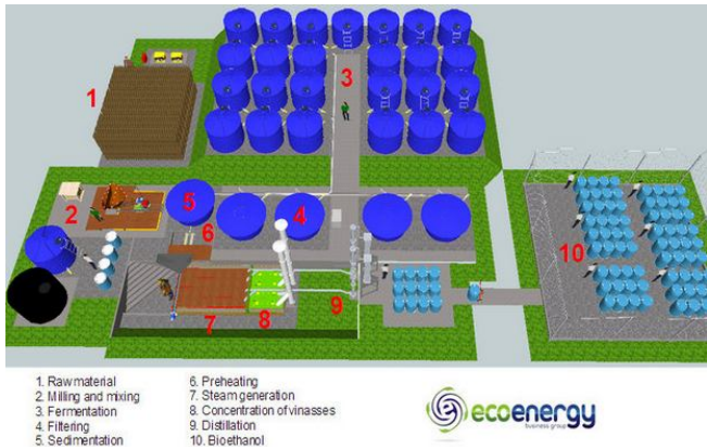
Figure 3: Typical plant layout for EMD
